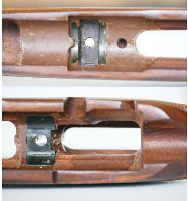
*Fore and aft bedding in the 97 DL stock showing epoxy bedded steel pillars.*
