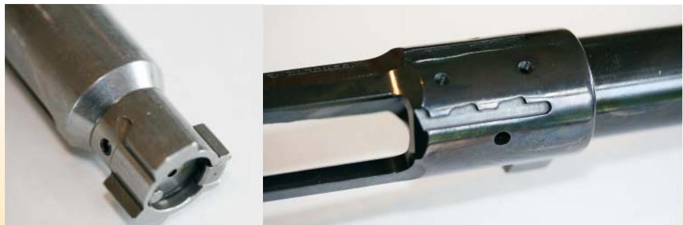
Left; The large bolt head with three locking lugs, slide extractor and ejector with plunger in the bolt face. Right: Integral base mounting system common to both models and also drilled and tapped for Weaver type bases.
